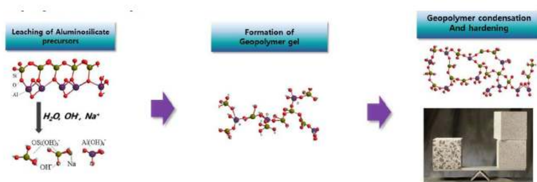
[Fig. 1] Schematic diagram of geopolymerization process.
